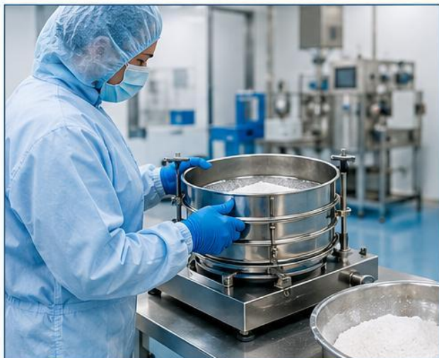
Figure 1. Sieving of pharmaceutical powder in a controlled manufacturing environment.
