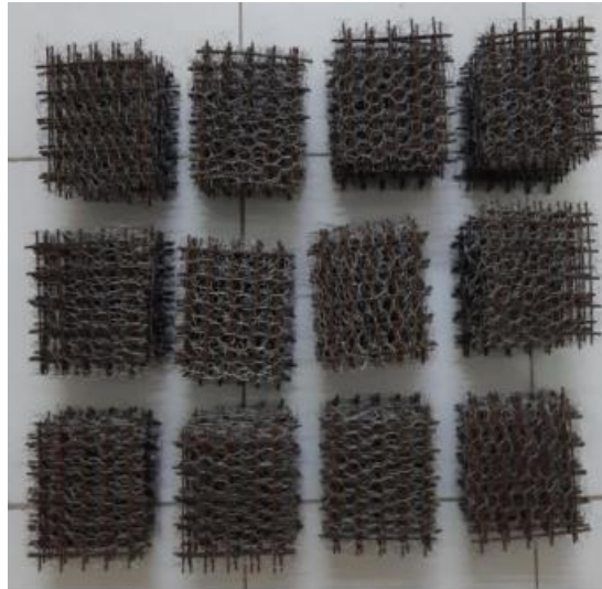
Figure 1 compressive strength- Steel mesh reinforcement
