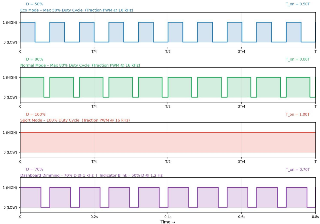
Figure 1: PWM Waveforms – Eco / Normal / Sport Modes & Peripheral Control
