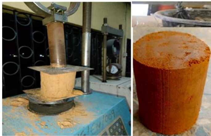
Figure 3. Compressive strength testing setup for stabilized lateritic blocks
