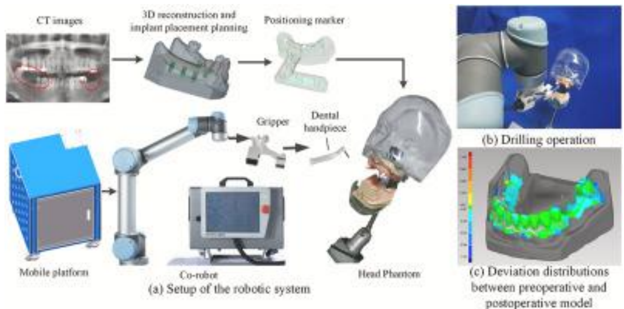
Figure 1 Dental Implantology AI-Based Assisting Robot Prototype Constructive Design.
