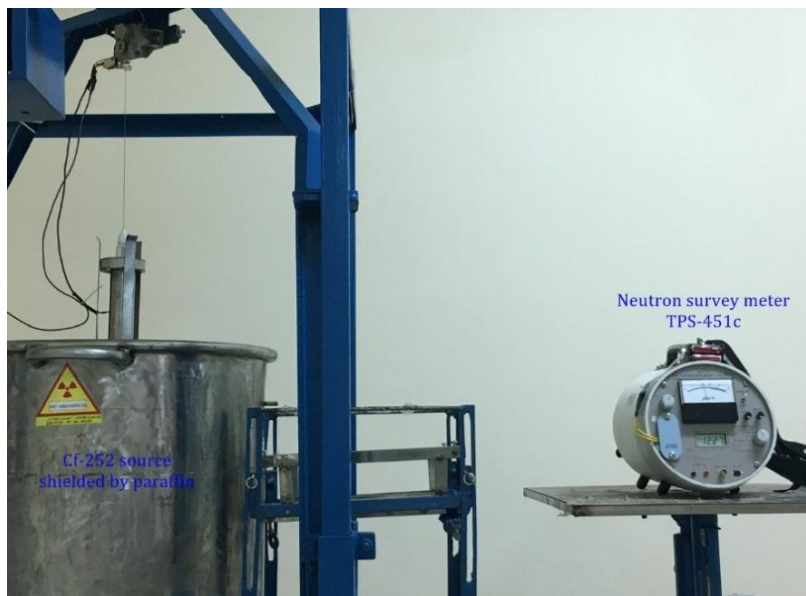
Figure 1. Experimental setup for determining neutron dose rate of Cf-252 source
