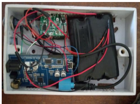
Figure 7: Internal construction of transmitter
