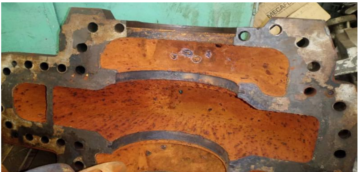
Figure 5: Effect of cavitation on the volute of a centrifugal pump
