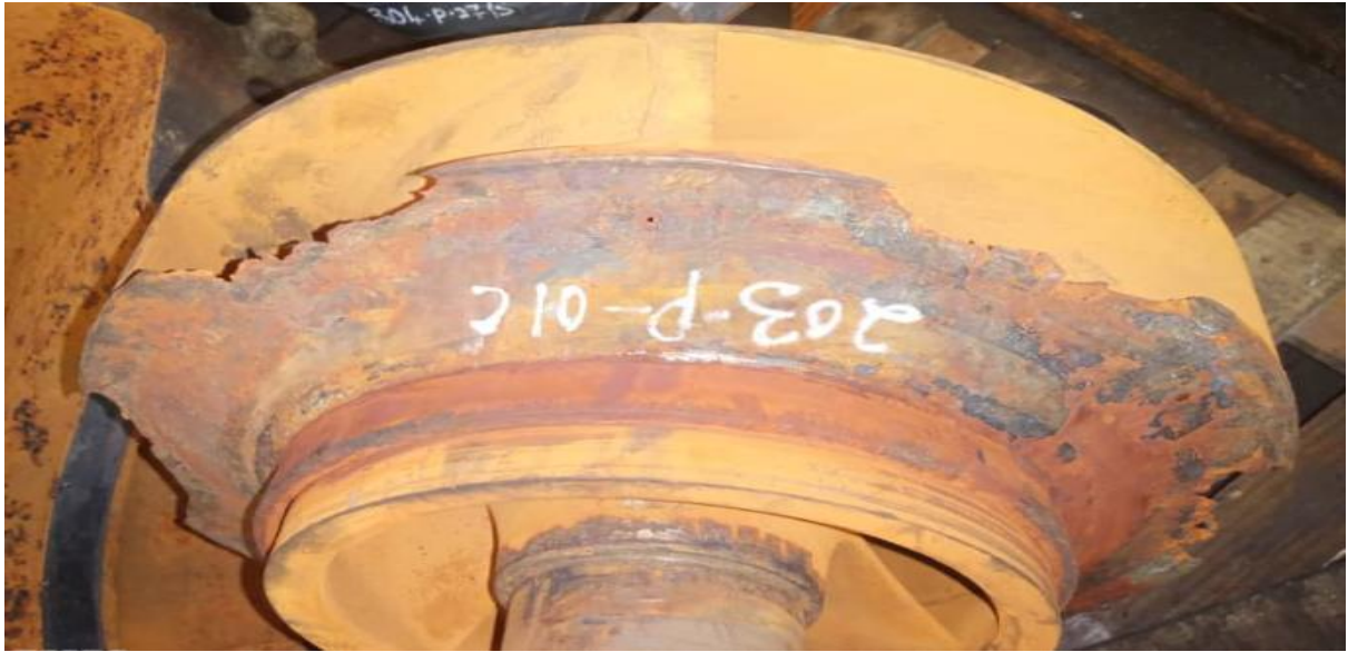
Figure 4: Effect of cavitation on an impeller of a centrifugal pump
