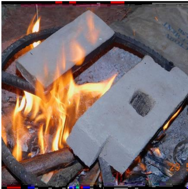
Figure 3 Fire resistance test-burning stage
