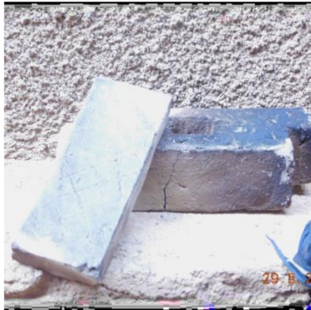
Figure 3 Fire resistance test- after burning process
